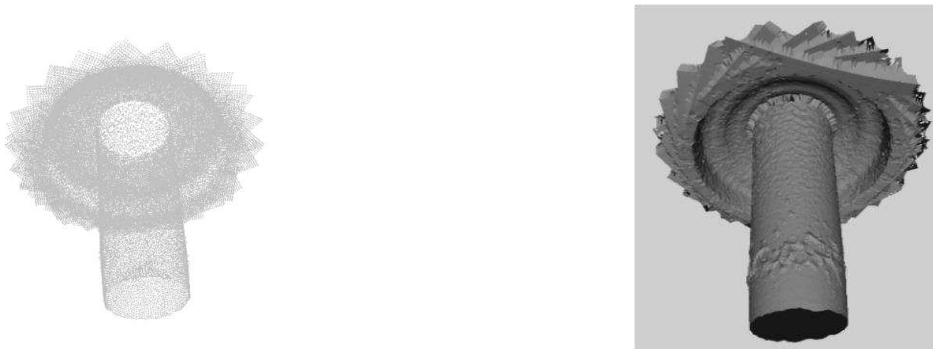
Figure 10 - 3D point cloud (left) and representation after mesh generation (right) obtained for simulated flexible joint.
