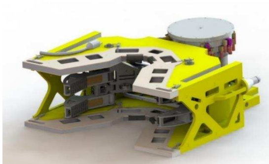
Figure 3 - Clamping system in detail.
